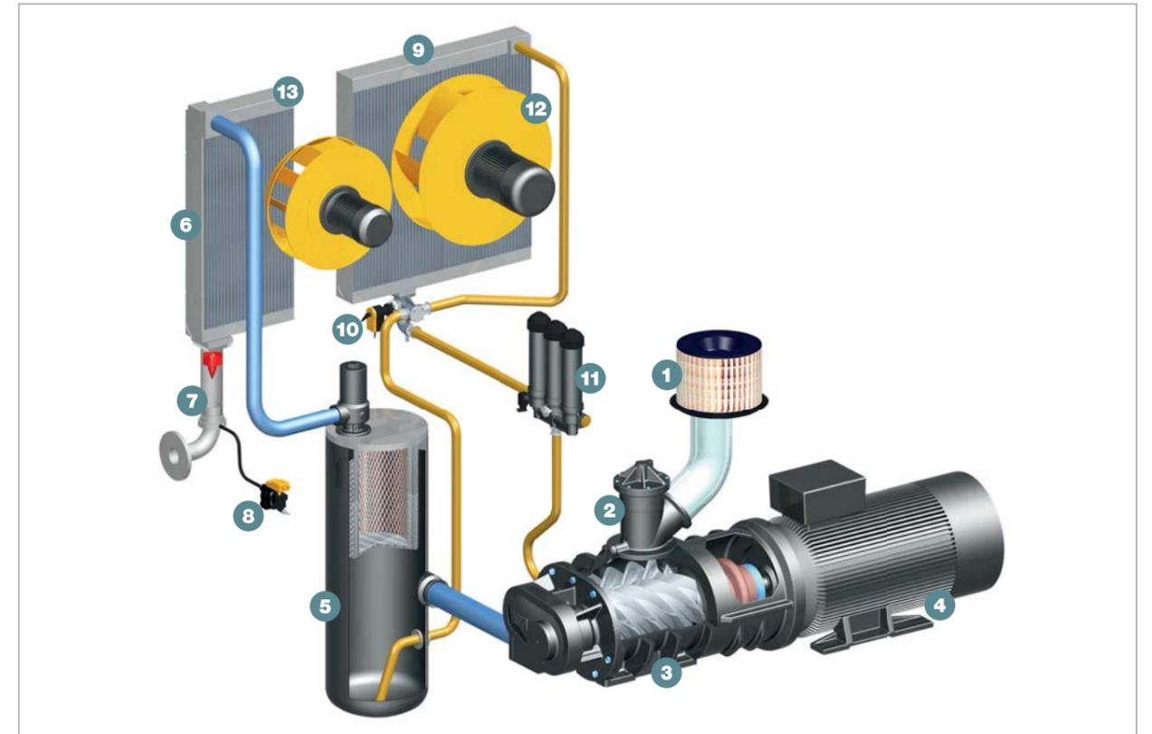
The rotary screw airend (3) is driven by an electric motor (4). The fluid injected primarily for cooling purposes during the compression process is separated once again from the air in the fluid separator (5). The integrated fan ensures cooling of the compressor package and also provides sufficient flow of cooling air through the oil cooler and compressed air aftercooler (6 and 9).
